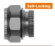
Corrosion-proof composite material. 310F\*045 composite shrink boot adapter fits MIL-DTL-38999 Series I and II connectors. Adapter has groove for lipped shrink boot. Antidecoupling mechanism provides audible detented coupling and prevents backoff under high vibration. Supplied as adapter only or as kit with shrink boot. Glass-filled high performance thermoplastic, silicone O-ring.
